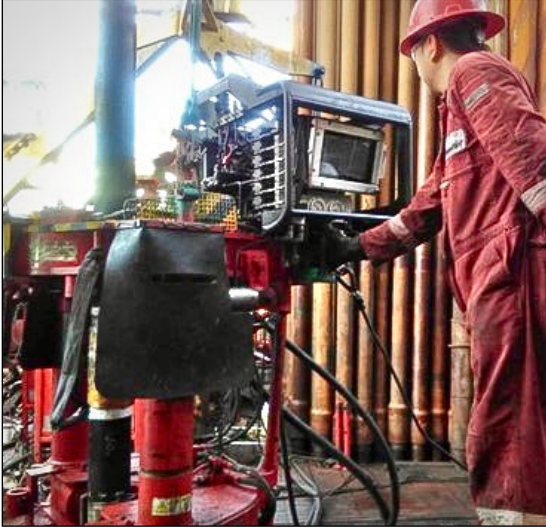
Weatherford tubular-running service crew operating the Vero conventional 7.6-30 system.
