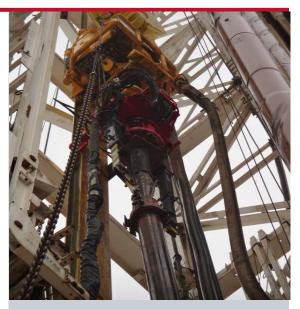
Weatherford's *OverDrive* casing running and drilling system with the *TorkDrive* tool enables the driller to rotate and push (or pull) the casing string while circulating, making it ideal for high-angle, extended-reach wells. The combined systems overcome drag on long strings of lateral pipe, mitigate wellbore sloughing, and efficiently handle other instability issues.
