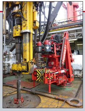
The Weatherford *TorkWrench* 10-100 iron roughneck provided up to 100,000 lbf-ft (135,582 N·m) of torque and a 40° wrenching angle for easy connection makeup and breakout. With a durable design that increases overall reliability, the *TorkWrench* 10-100 outperformed previous iron roughnecks, which had multiple failures and high maintenance costs.
