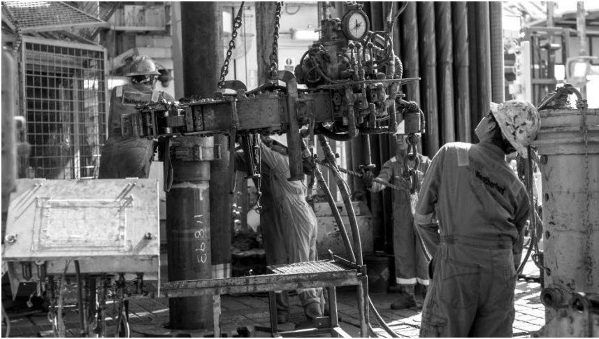
The Weatherford 14-50 high-torque casing tong is lightweight and easy to operate, which saves time and enhances personnel safety.
