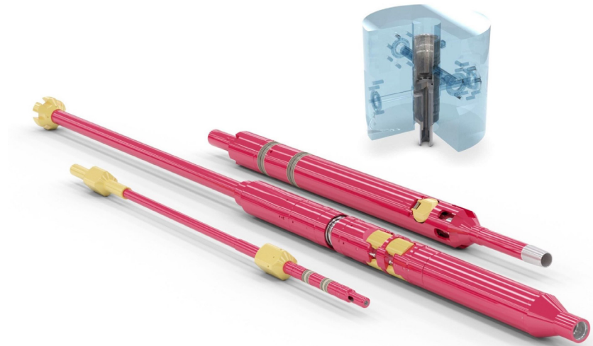
The IGLS system is separated into upper and lower completion components. The upper completion has an Intermediate spool and concentric hanger at the wellhead, along with jointed tubing, and a seal stinger with pumpout plug. The lower completion includes a dual flow hanger / suspension hanger, a dual-flow safety valve, and injection valve.
