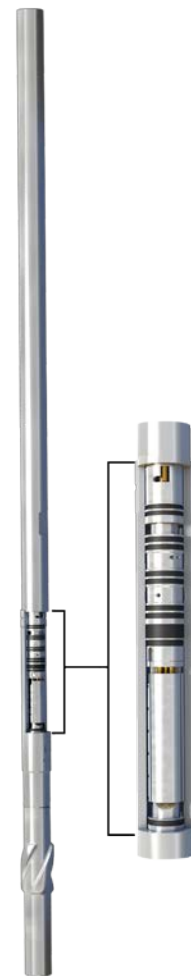
Part of the HEL MWD system, the Weatherford bore and annular pressure sensor uses quartz transducers to measure downhole temperature and pressure within \pm 7.5 psi (0.052 MPa).
