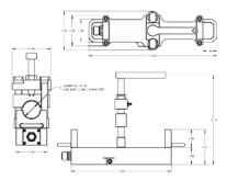
The hookload/weight-on-bit sensor converts deadline tension to hookload or WOB measurements.
