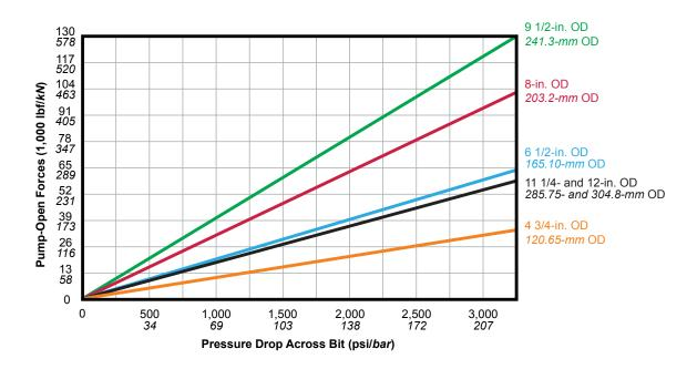
Pump-open force is created by pressure drop across the bit. The pump pressure creates a reaction force in the tool that tries to force it open. Reduce the pump to idle before attempting to jar.
