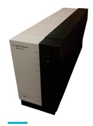
The quad-column chromatograph uses a thermal conductivity sensor to clearly separate peaks. which enables discrete analysis of previously undetectable combinations of gases.
