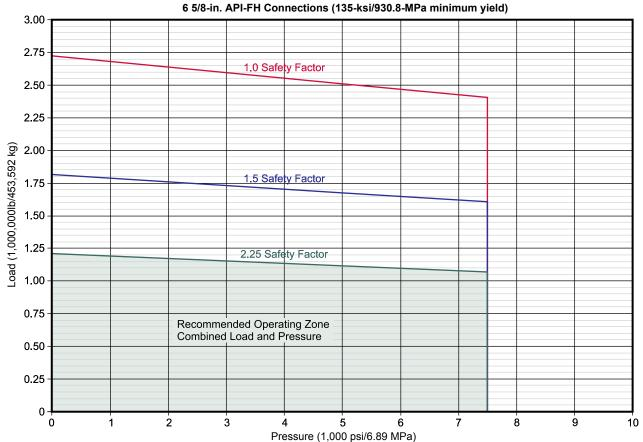
Weatherford TDH Combined Tension and Pressure 5/8-in, API-FH Connections (135-ksi/930.8-MPa minimum viel
