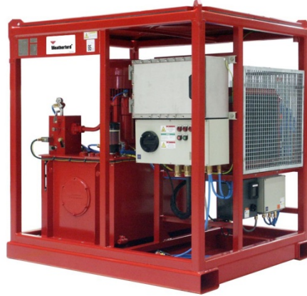
Left: A type-2EW, 22-kW electrohydraulic power unit for use in Zone-1 environments Right: A 55-kW electrohydraulic power unit for use in Zone-1 environments
