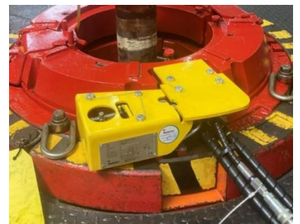
The StringGuard indicator can be easily adapted to existing designated spiders.
