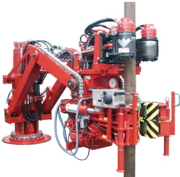
The photo at the left shows the TorkWrench 10-145 iron roughneck with the PowerArm 2.1 tong-positioning device.
