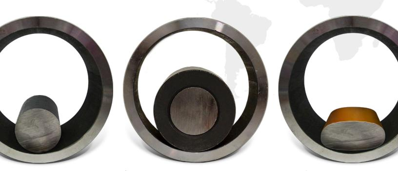
**COROD eliminates the need for couplings, centralizers, and rod guides** to maximize production flow by creating a larger annular space between the production tubing and the rod string.
