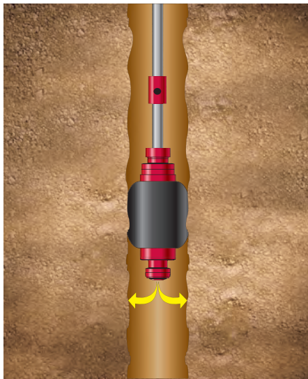
The IPP packer can isolate specific sectors to perform injectivity tests.
