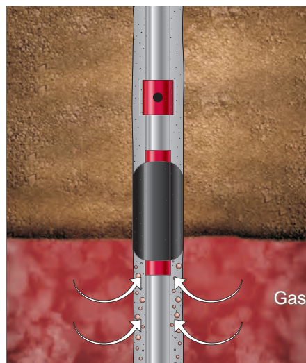
Position the ACP system just above the gas zone to isolate the gas and eliminate channeling.
