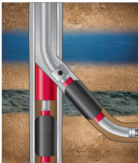
The ACP system can be run through a milled window. The packer is inflated and a cement job is performed above the packer to isolate the producing zone.
